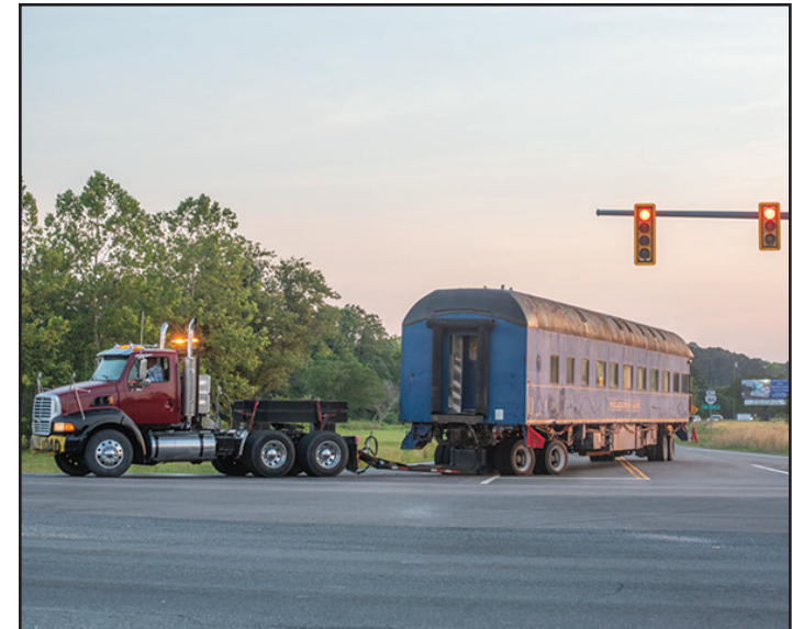
Timbers prevent solid-rubber wheels from damaging the soft shoulder of the road as the rail car inches across Cassatt Parkway in Cape Charles.
