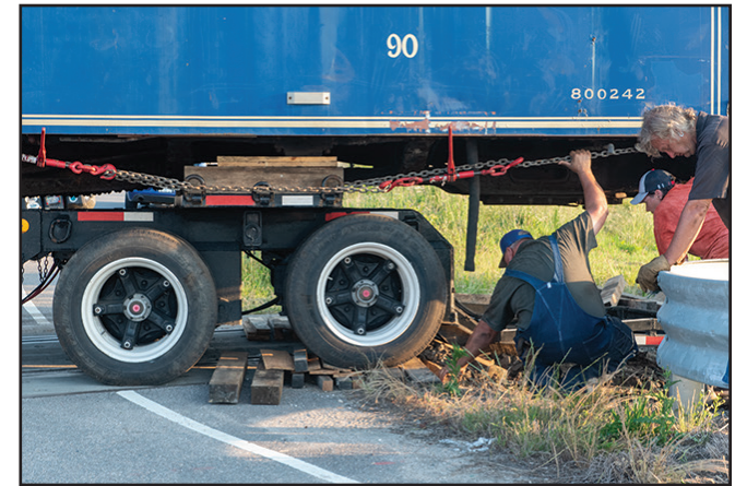
Timbers prevent solid-rubber wheels from damaging the soft shoulder of the road as the rail car inches across Cassatt Parkway in Cape Charles.
