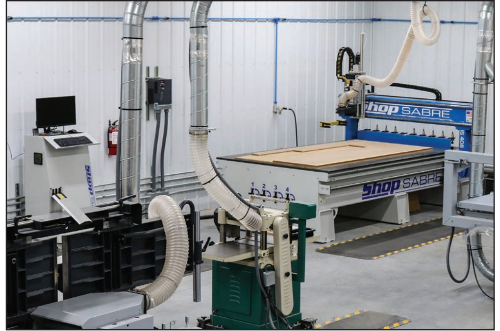
The ShopSabre computer numerical control or CNC router is made to order in America. The computer that controls the machine is shown at left. Submitted Photo.
