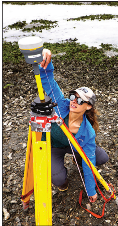
Clockwise from top: (1) Cora Johnston and Kinsey Tedford count and measure oysters within a quadrat (the white rectangular tool in the photo) on top of a reef. The data will inform them about oyster survival and growth rates. (2) Tedford uses an RTK (real-time kinematic) GPS (global positioning system) to measure elevation across the oyster reefs. Photos by Aileen Devlin. (3) Tedford kneels next to an oyster reef on Hog Island. Photo by Rachel Smith.
