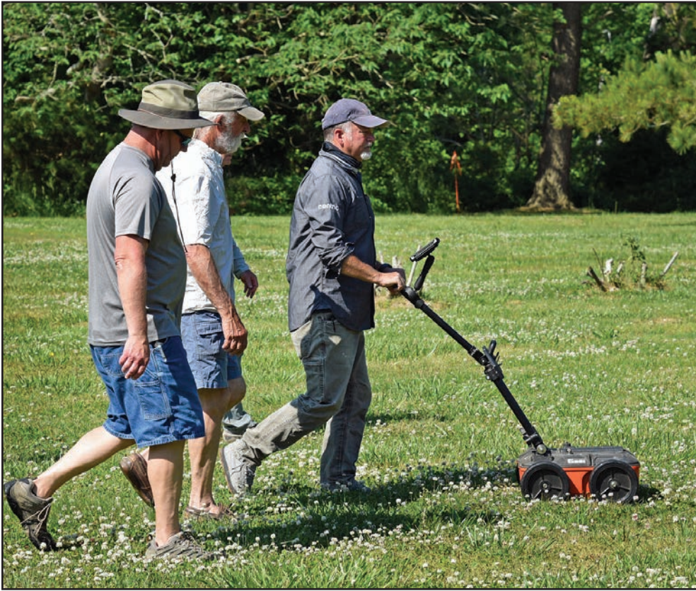
Jamestown archaeologist David Givens pushes a ground-penetrating radar unit across the foundation site of the Assawaman Church that was built in 1680. John “JD” Barnes, left, and David Bundick, center, were among a dozen volunteers who recently helped survey the area.
