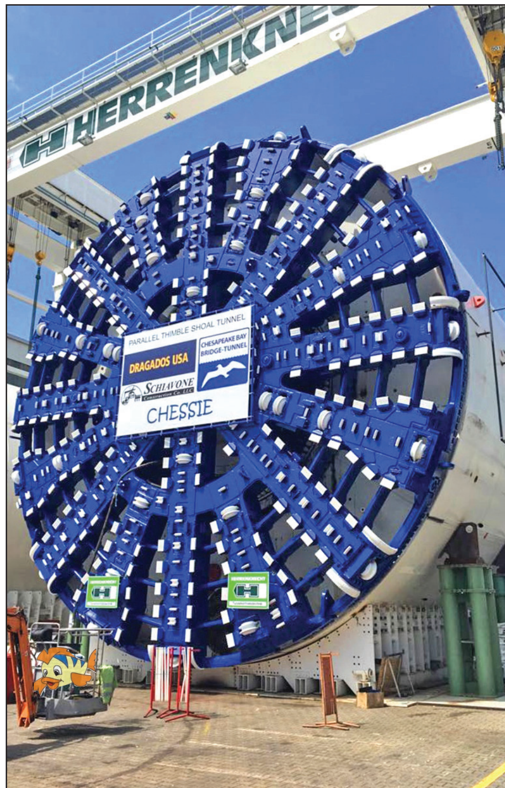
The image above shows “Chessie,” the tunnel boring machine manufactured in Germany, which will be used during construction of the parallel Thimble Shoals tunnel of the Chesapeake Bay Bridge-Tunnel. Photo courtesy of the CBBT.
