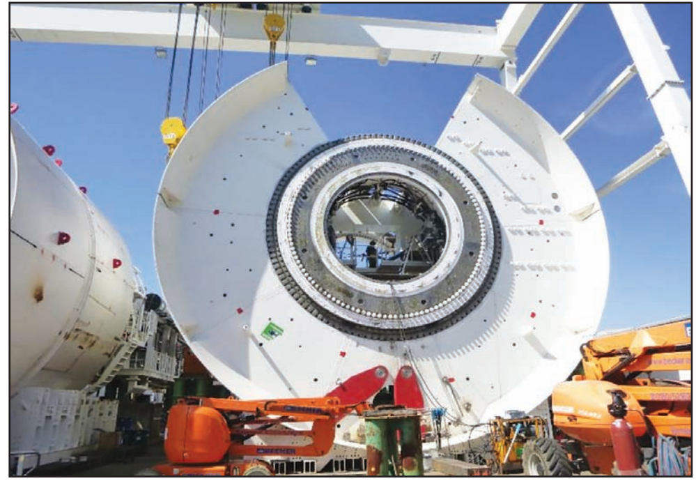
Photo courtesy of the Chesapeake Bay Bridge-Tunnel Chessie, the newly named tunnel boring machine under construction in Germany.
