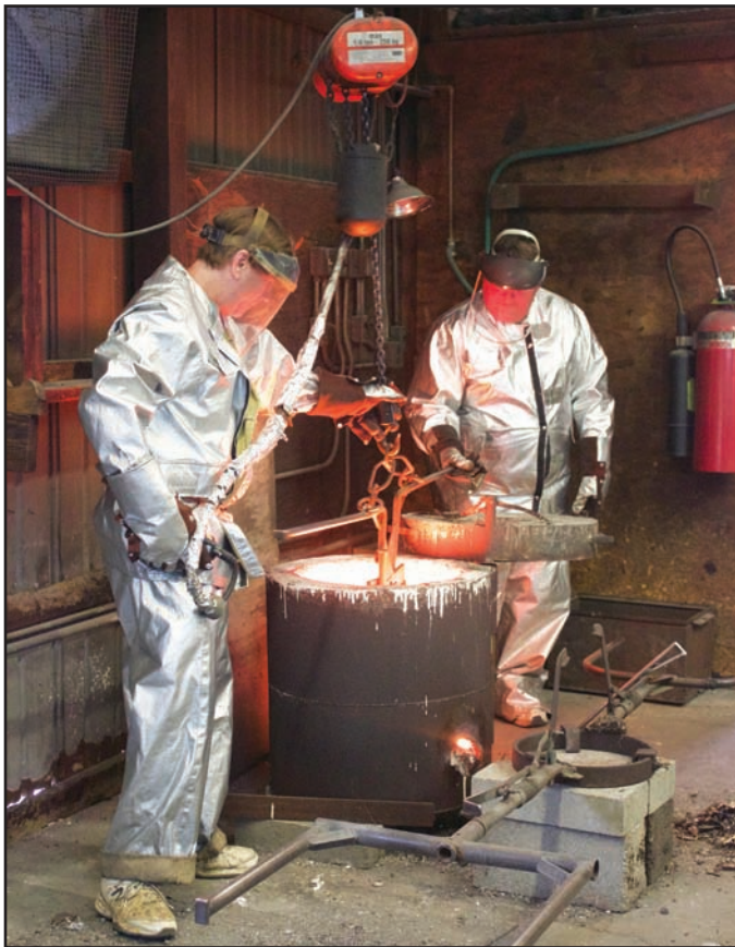
Workers pour and mold what will become the Unity Eagle.
